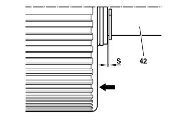
f) Test and set the axial play of the K3 multi-disk clutch on the output shaft! Which measuring instruments do you need? What is the axial play set with?
