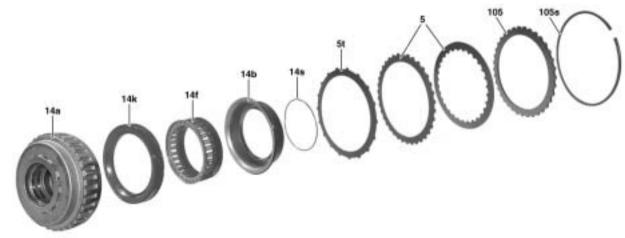
d) Measure the clearance of the K1 clutch and set the play correctly!
